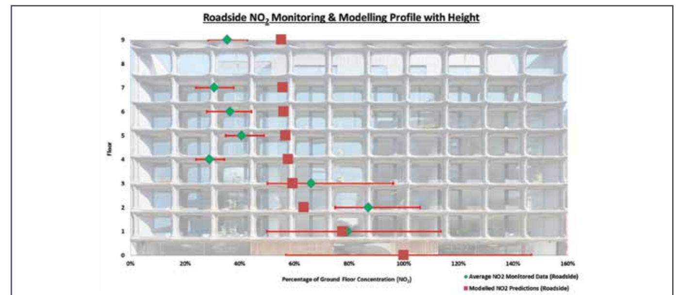
Figure 10: Comparison of roadside NO 2 diffusion tube monitoring and typical modelled concentration profile for NO 2 . The green points indicate the average monitored NO 2 concentration for each floor and the red bars indicate the minimum (left) and maximum (right) NO 2 concentrations measured at each floor. The red points indicate the modelled NO 2 concentrations predicted at each floor
