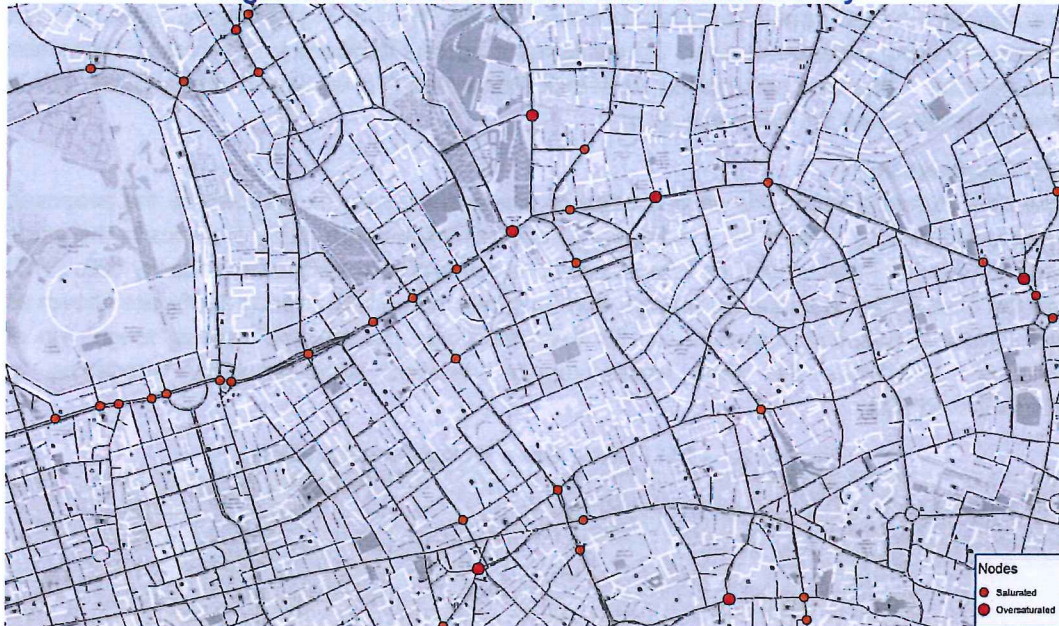
Figure 23 – AM Future Closure Model Junction Delay
