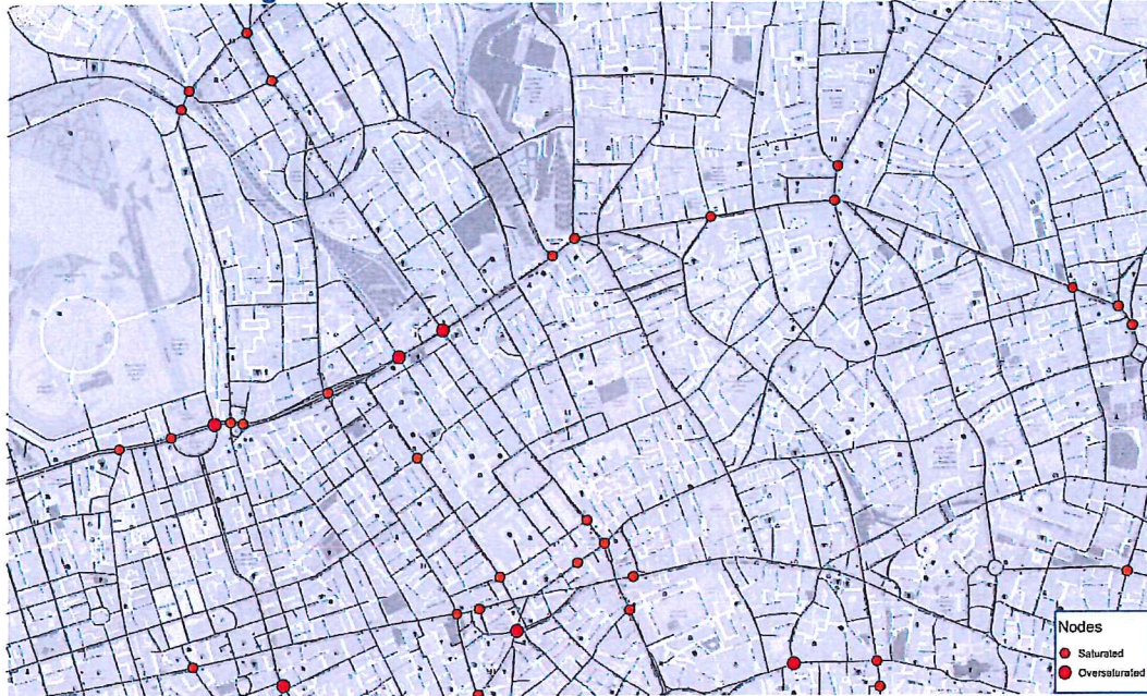
Figure 25 – PM Future Closure Model Junction Delay
