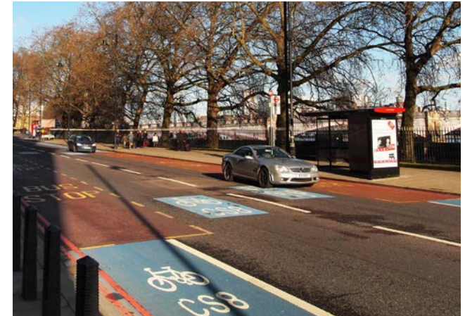
Lane ends at bus stop cage, with cycle symbols marked around cage
