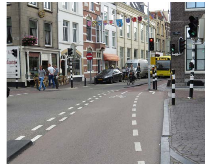
Cyclists in Utrecht using the crossing to turn left are directed to wait on the right, to allow ahead cycle movement to continue
