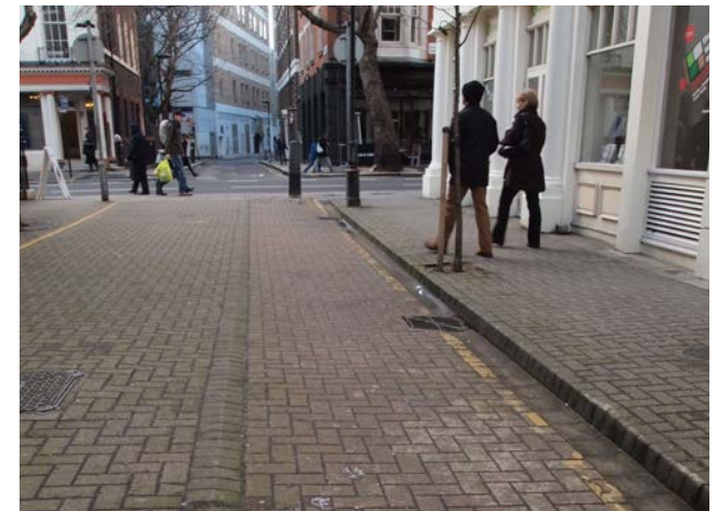
Separation by level difference in areas closed to motorised traffic – (left) Separated track and footpath in Copenhagen and (right) Steatham Street, Camden
