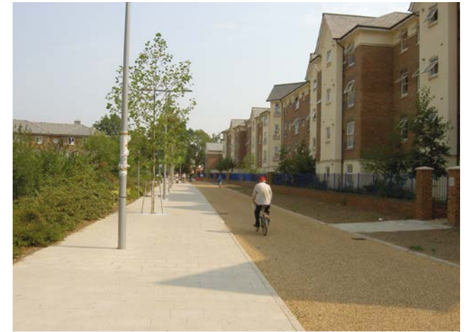
Separation by level difference in areas closed to motorised traffic – Skerne Walk, Kingston
