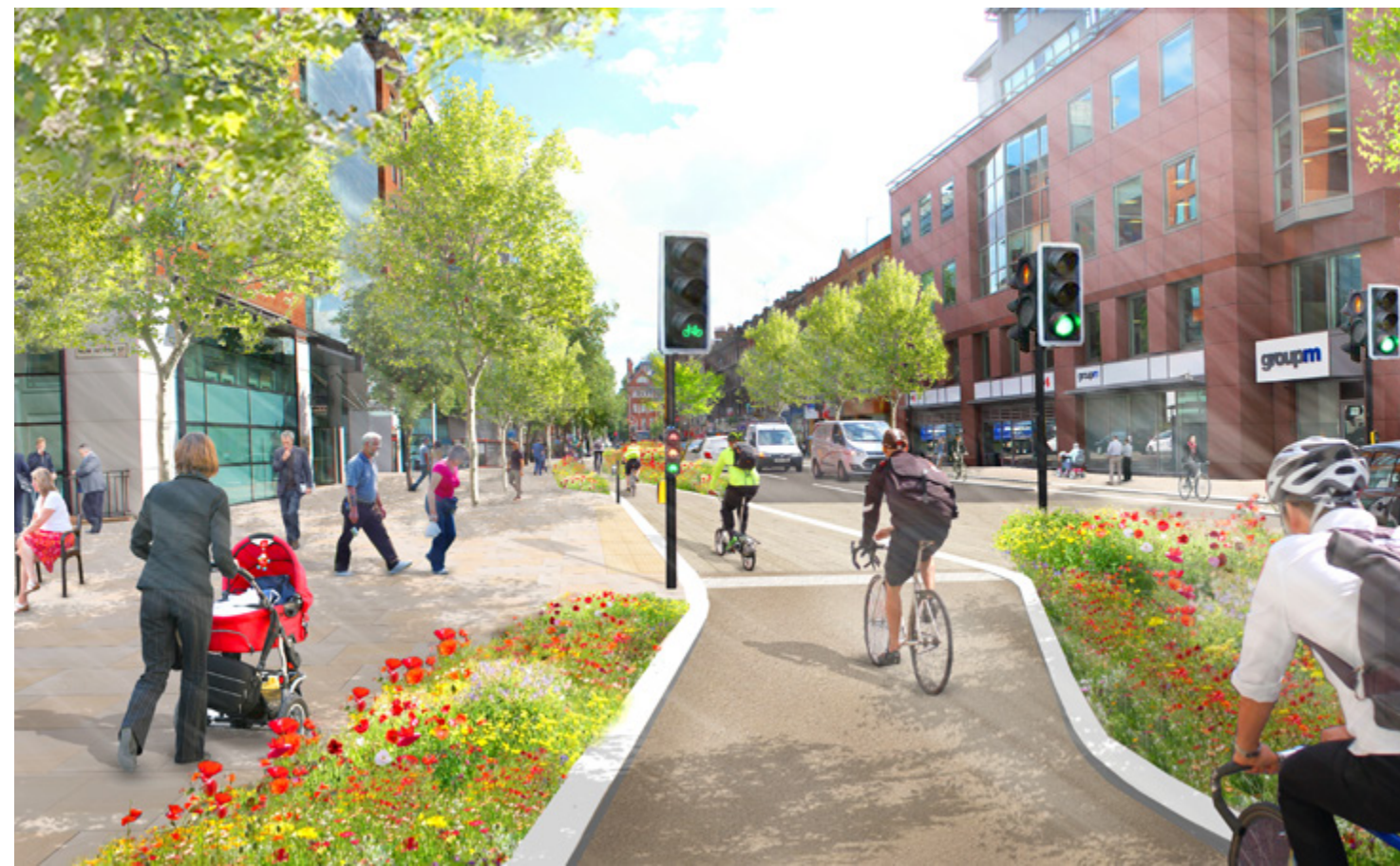
Theobalds Road Opportunity for a new identity, reducing vehicular lanes, with segregated cycle lanes, floating bus stops. In the high streets areas, the public realm can support local uses, introducing spill-out space, incidental seating and planting, as appropriate. North south pedestrian connections across the street can be reinforced, through measures such as raised tables, wayfinding, de-cluttering, art and material changes.
